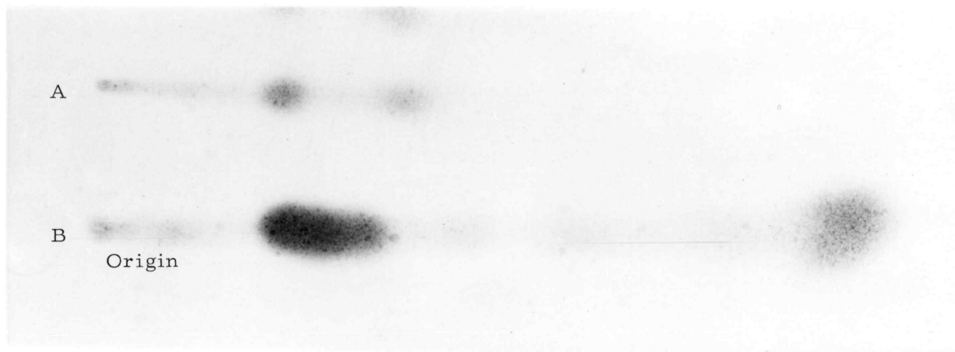
Figure 12. Preparative layer chromatography of prenol sample. A. Prenol sample B. Standards, left to right, cholesterol-farnesol, and squalene.
